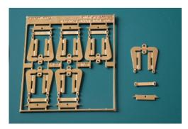
After drilling all the holes, cut the components from the fret.
