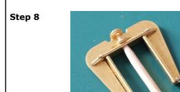
Insert the top tab and solder all the joint and fold lines. A cocktail stick will help align the holes and hold the parts.
