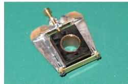
The complete hornguide is now ready for installation in the chassis. Repeat steps 4 to 13 for the remaining hornguides.
