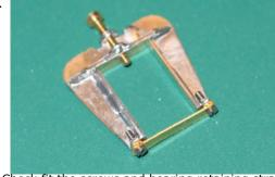
Check fit the screws and bearing retaining strap.
