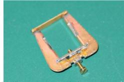
The top 'shelf' is used to ensure the hornguides are in line in the chassis so any excess solder should be removed from the adjacent seam. At this stage you can remove the etching cusps from any visible edges, if you wish to do so.
